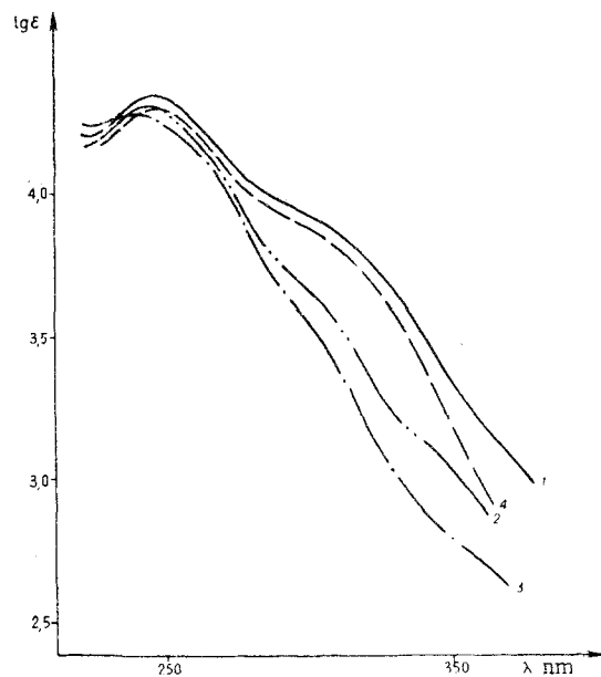
Fig. 2. A study of the cleavage of the indandione ring by UV spectra (concentration 10^{-4} M): 1) N-ethyl-N-(2-phenyl-1,3-indandion-2-yl)thiourea in concentrated \text{H}_2\text{SO}_4 ; 2) the same in 85% \text{H}_2\text{SO}_4 ; 3) the same in 65% \text{H}_2\text{SO}_4 ; 4) 4-(o-carboxyphenyl)-1-ethyl-5-phenyl-2-imidazolethione in concentrated \text{H}_2\text{SO}_4 .
